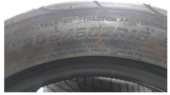
Here, the **205** represents the tire width in millimeters. The **50** represents the tire's sidewall aspect. This number is a percentage of the width. In this case this sidewall is 50% of the width of the tire. The final number is the **R15** (in some cases, such as this, ZR is used to indicate this is a performance tire). This represents the diameter of your rim/wheel in inches.
